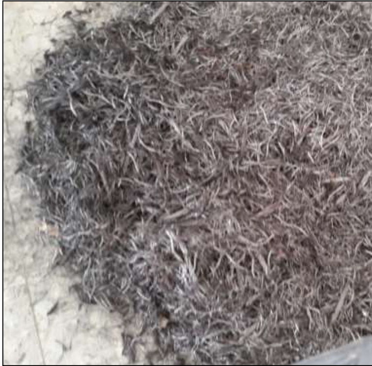
Figure 3.4: Steel Fibers used in mixes
